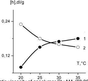
Figure 1. Characteristic viscosity of copolymer St : MA (80:20 % by weight) as the function of solution temperature. Solvents: 1 – DMFA, 2 – toluene.
