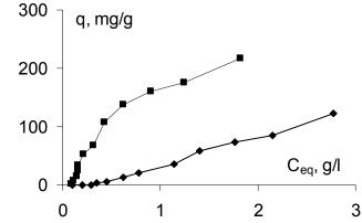
Figure 1. Sorption isotherms of the silanol derivatives of leonardite HA onto silica gel. ■ - CHS-APTES-100; ♦ - CHS-APTES-20
