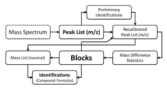
Figure 1. Spectrum interpretation workflow using *Transhumus* software. Boxes show data tables, arrows represent the relation "is needed to obtain" between data. The "Mass Spectrum" box is dashed because peak picking means are not included in *Transhumus*.
