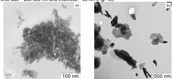
Fig. 1. Transmission electron microscopy images of feroxyhyte (δ-FeOOH) nanoparticles synthesized under different conditions: a) in the presence of HS, b) without HS.
