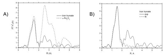
Figure 1. FT of EXAFS spectra of iron humate in comparison with standard  $\alpha$ -Fe<sub>2</sub>O<sub>3</sub> (A) and first shell approximation of local neighborhood of Fe (B).
