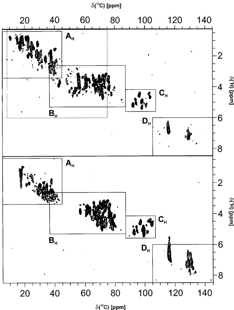
Fig. 5. Heteronuclear single quantum coherence (HSQC) nuclear magnetic resonance (NMR) spectra of a peat fulvic acid (FA) (bottom) and humic acid (HA) (top) with sections of chemical shift indicated in Table 5; the dotted box corresponds to the range of chemical shifts shown in Fig. 6.
