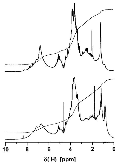
Fig. 1. The  $^1\text{H}$  nuclear magnetic resonance (NMR) spectrum of the peat fulvic acid (FA) (top) and humic acid (HA) (bottom).
