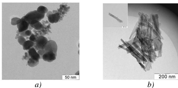
Figure 1: TEM images of  $\delta$ -FeOOH – a) and  $\gamma$ -Fe<sub>2</sub>O<sub>3</sub> – b)
