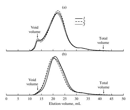
**Fig. 1.** Gel chromatograms of HA preparations obtained by sequential alkaline extractions from (a) soddy-podzolic soil under forest and (b) typical chernozem of the experimental treatment with permanent black fallow since 1964 (here and below: (1)-(3) alkaline extraction numbers); all chromatograms are normalized to the unit area.
