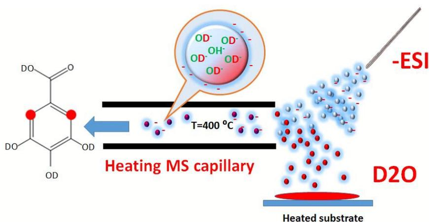
**Fig. 1** The design of the in-ESI source H/D exchange experiment. The charged droplets are produced by the ESI source; they pass through the D<sub>2</sub>O-saturated region, enter heated capillary and evaporate producing the gas phase ions. During this transport the charged droplets interact with D<sub>2</sub>O containing trace amounts of hydroxyls, and exchange protium against deuterium. Red dots designate C-H sites capable of keto-enol tautomerism, which have undergone labeling.
