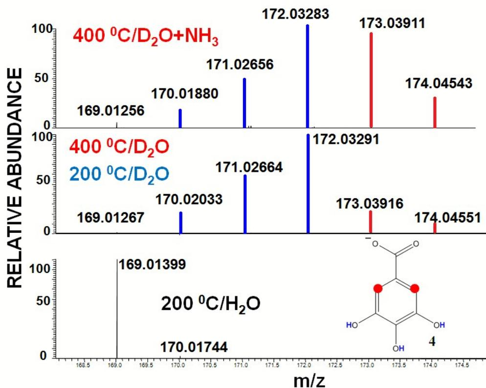
**Fig. 3** In-ESI source H/D exchange series of gallic acid (**4**) in the absence and presence of ammonia. The peaks corresponding to labile and backbone deuterium are highlighted with blue and red color, respectively. Red dots in the structural formulas designate the feasible sites for deuteration in accordance with keto-enol tautomerism.
