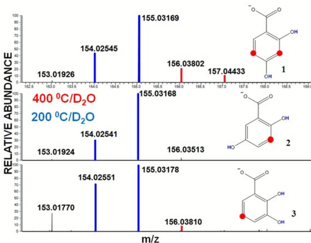
**Fig. 2** In-ESI source H/D exchange series of 2,4-DHB, 2,5-DHB, and 2,3-DHB at 200 °C (blue lines) and 400 °C (additional peaks are colored in red). Red dots in the structural formulas designate the feasible sites of deuteration in accordance with keto-enol tautomerism and mesomeric substituent effects in the aromatic ring.
